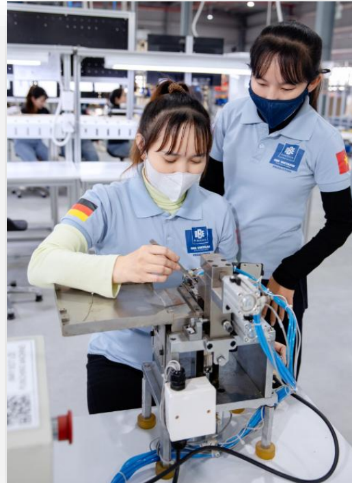
Q3 2025 Welding & Soldering of hinges on wire cores
